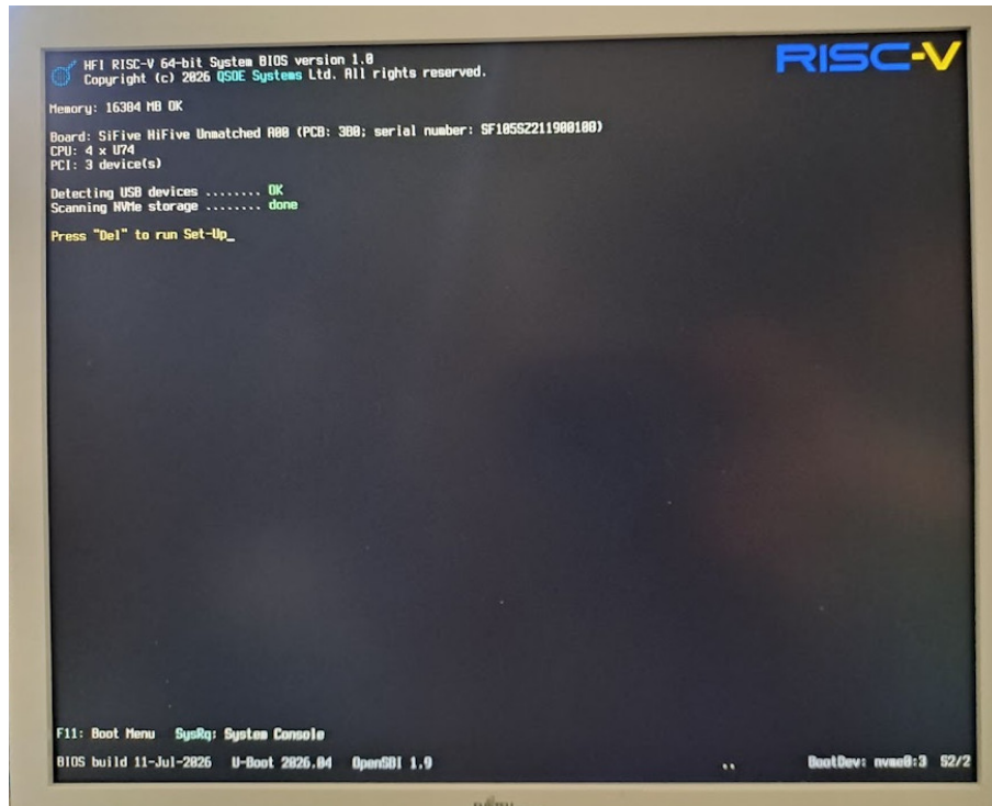
Figure 2. HFI's power-on identity screen: board inventory, storage and USB enumeration, a system console, boot menus---rendered by a discrete GPU on a RISC-V board, photographed on a period CRT.
